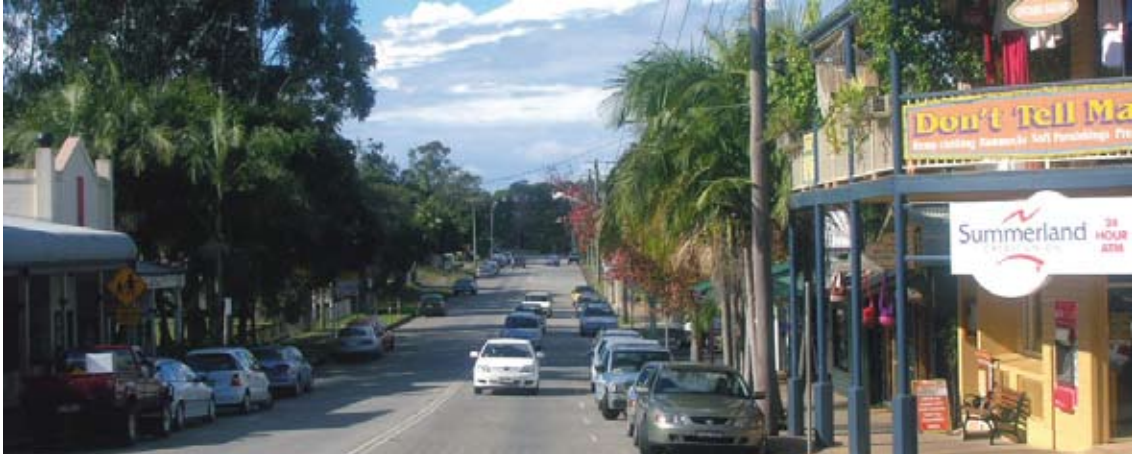
Formal main street with parallel parking either side; awnings extend intermittently along kerb edge with a consistent building setback; buildings without awnings provide opportunity for planting along wide footpaths
