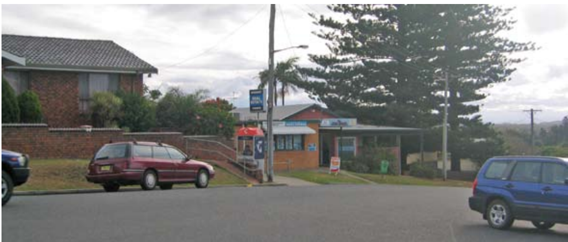
Asymmetrical, wide carriageway with formed kerb and gutter, angle parking to one side of the street and parallel parking to the other side, accommodating low key commercial activity within a residential street
