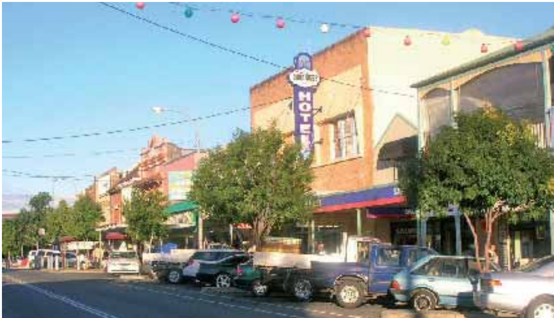
Commercial centre street with formal carriageway and angle parking with parallel parking to opposite side, some street planting and intermittently covered footpaths
