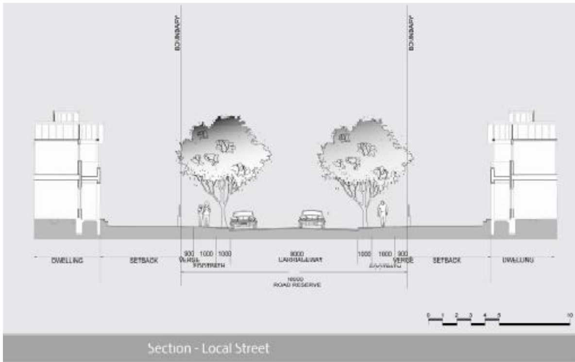
Figure 6-6 Local road – typical cross-section
