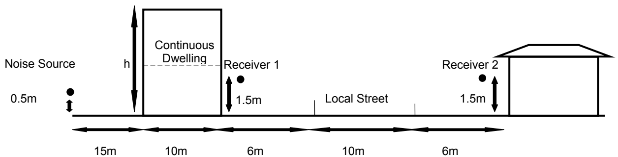
Figure 8 Continuous dwelling acting as noise barrier
