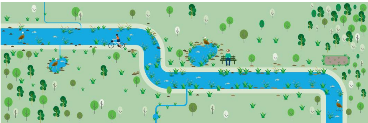
Figure 12: Multi-functional stormwater infrastructure areas will co-locate wetlands, creeks and open space to meet water management needs and provide recreation, amenity and urban cooling
